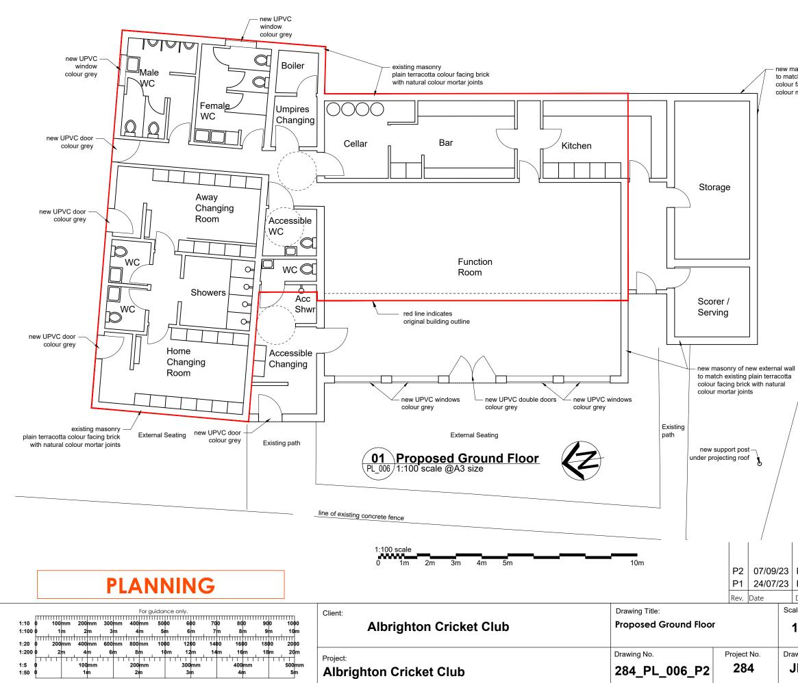
new masonry of new external wall to match existing plain terracotta colour facing brick with natural colour mortar joints
